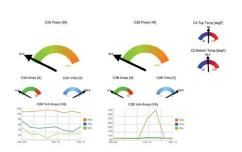
The EMX management tool for all wire-free monitoring units captures, analyses and reports power and environmental data via dynamic charts, dashboards and diagrams.
