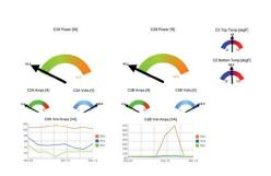
The EMX management tool for all wire-free monitoring units captures, analyses and reports power and environmental data via dynamic charts, dashboards and diagrams. allows for direct placement of the temperature sensors inside the PDU cabinets. The module itself is battery powered, so no external power source is needed. Since it is non-intrusive it can be installed within minutes and without isolating the PDU.
